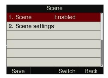
3. When under the **Multiple scene**, you can press **the down** key enter to the **Scene settings**, then user can enable the **Scene1**, **Scene2** or **Scene3**.
