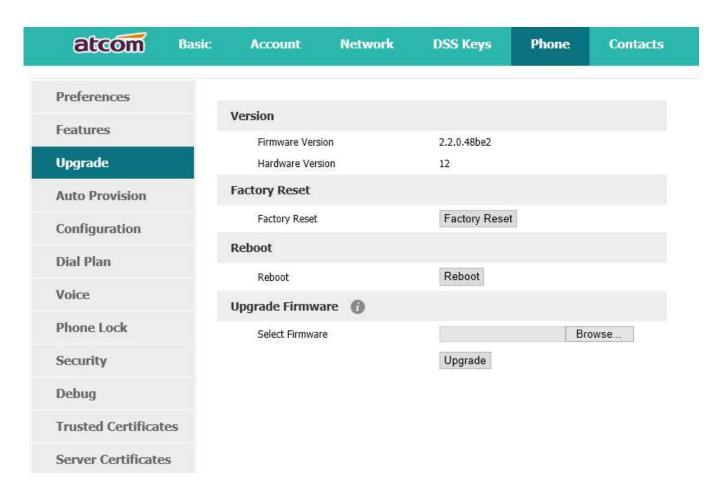
Before upgrading the firmware of phone, users are suggested to check the version of current firmware. Click the button "Choose file" to select the target local file and click "Upgrade" to process upgrading, this will cost a couple of minutes. And after reboot, the phone will be upgraded successfully.
