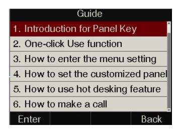
Press the Down key or the number can enter the corresponding guide feature.
