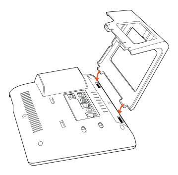
B. Press the other side joints into the slot according to the direction of the arrow:
