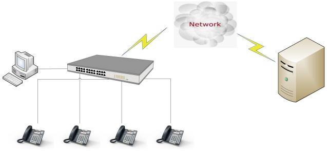
Connect LAN port to PC with Ethernet cable, or connect Rainbow2 to a switch/router which is in the same network as your PC. It uses DHCP mode by default, and you can review its current IP address
